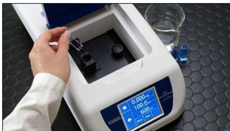
Figure 3: SPF protection activity test using spectrophotometer
