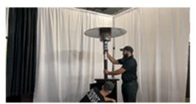
(2 - person lift) Raise the heater, apply the saftey bar underneath, and tighten the main screw.
