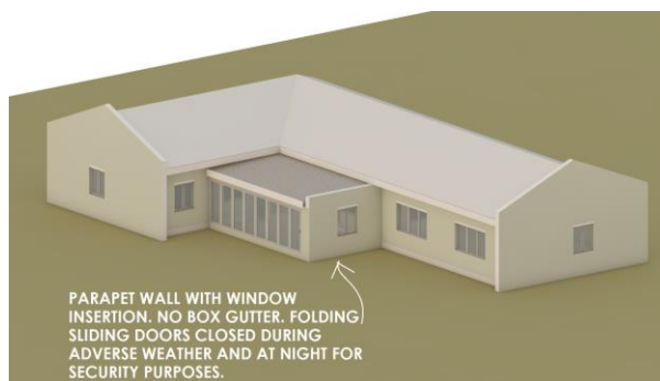
Above: 11.3.1 Example of parapet wall and window insertion. Below: 11.3.2 Patio to still function as open patio.
