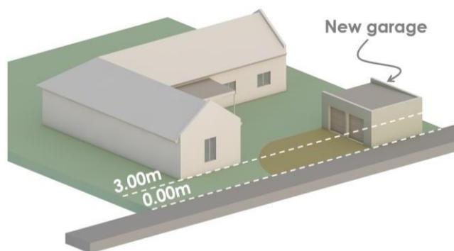
Above: Example of side entering garage layout, with driveway forming parking space in front of garage. Note: street building line of 3.0m for dwellings, 4.0m for garages.
