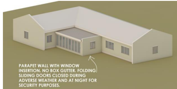
Above: Clause 11.4: Example of parapet wall and window insertion.
