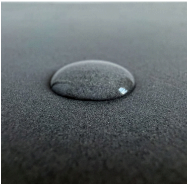
FIG. 3 — HYDROPHOBIC SURFACE (ZERO MOISTURE ABSORPTION)
