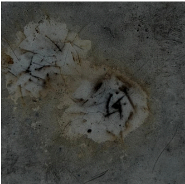
FIG. 2 — VERTICAL BURN TEST (ZERO MELT/DRIP)
