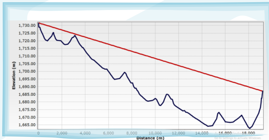
Figure 5: Line A Hydraulic Grade Line at Scenario 2
