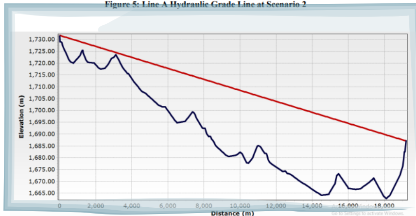
Figure 5: Line A Hydraulic Grade Line at Scenario 2
