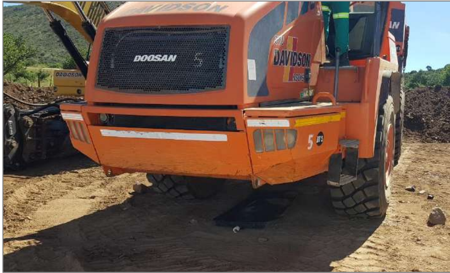
Figure 3: Drip tray being placed under vehicles when stationary.
