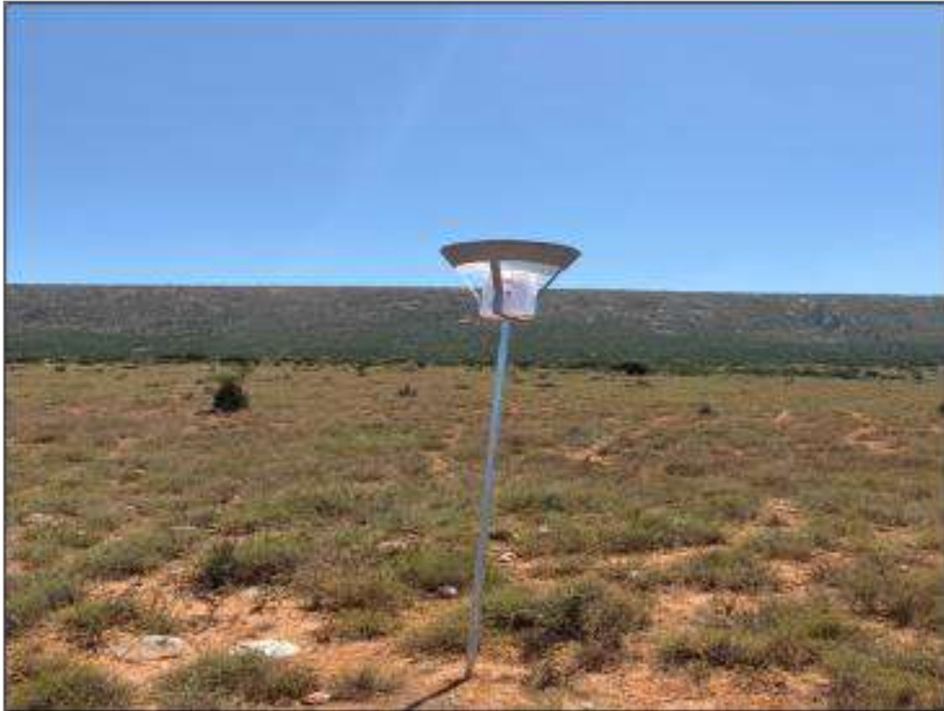
Figure 3: Dust bucket installed for dust monitoring. (C. Billing, 2023)
