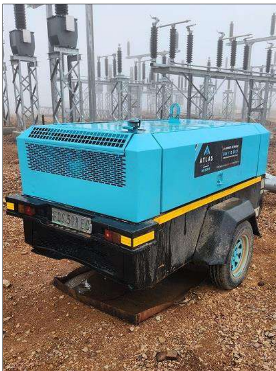
Photo 13a: Drip trays observed in use for mobile generators on site.
