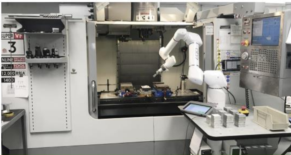
OB7 LOCATED WHERE IT CAN REACH THE WORK, THE DOOR AND THE "START" BUTTON
