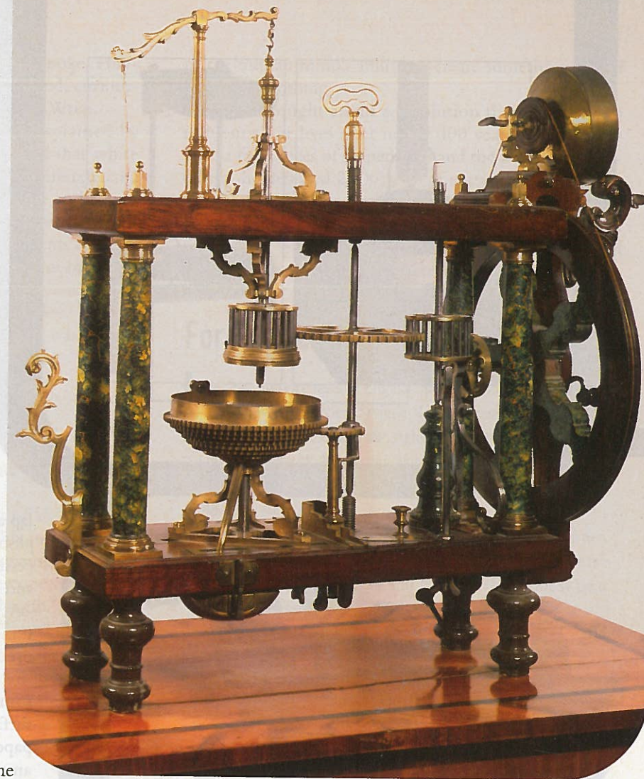
After its importance to science became well known, lens grinding became fashionable. Elaborate lathes, like this one made by Andrea Frati in the 18th century, graced the parlors of wealthy nobles.
