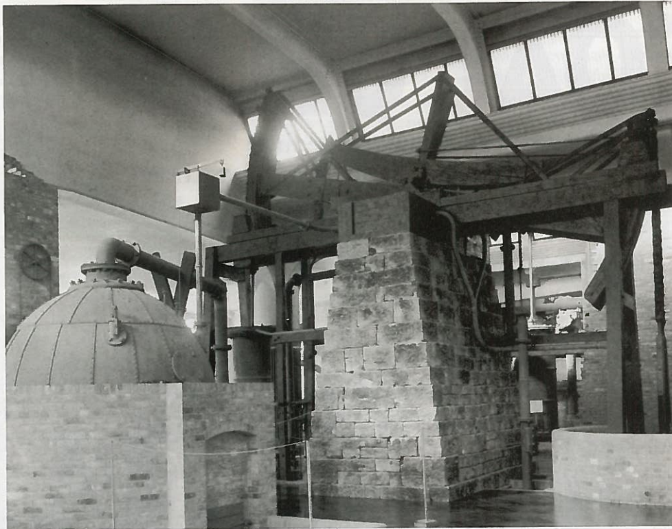
Fairbottom Bobs, a Newcomen steam engine recovered from a mine site in Lancashire, England, was acquired in 1930 by the Henry Ford Museum, which says it is possibly the oldest extant steam engine in the world.
