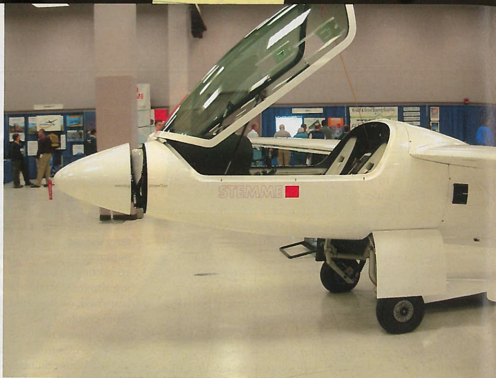
The propeller blades of the S10-VT made by Stemme AG fold up inside the nose cone when they stop turning. The nose cone can be retracted to streamline the fuselage. The blades are held open by centrifugal force.
