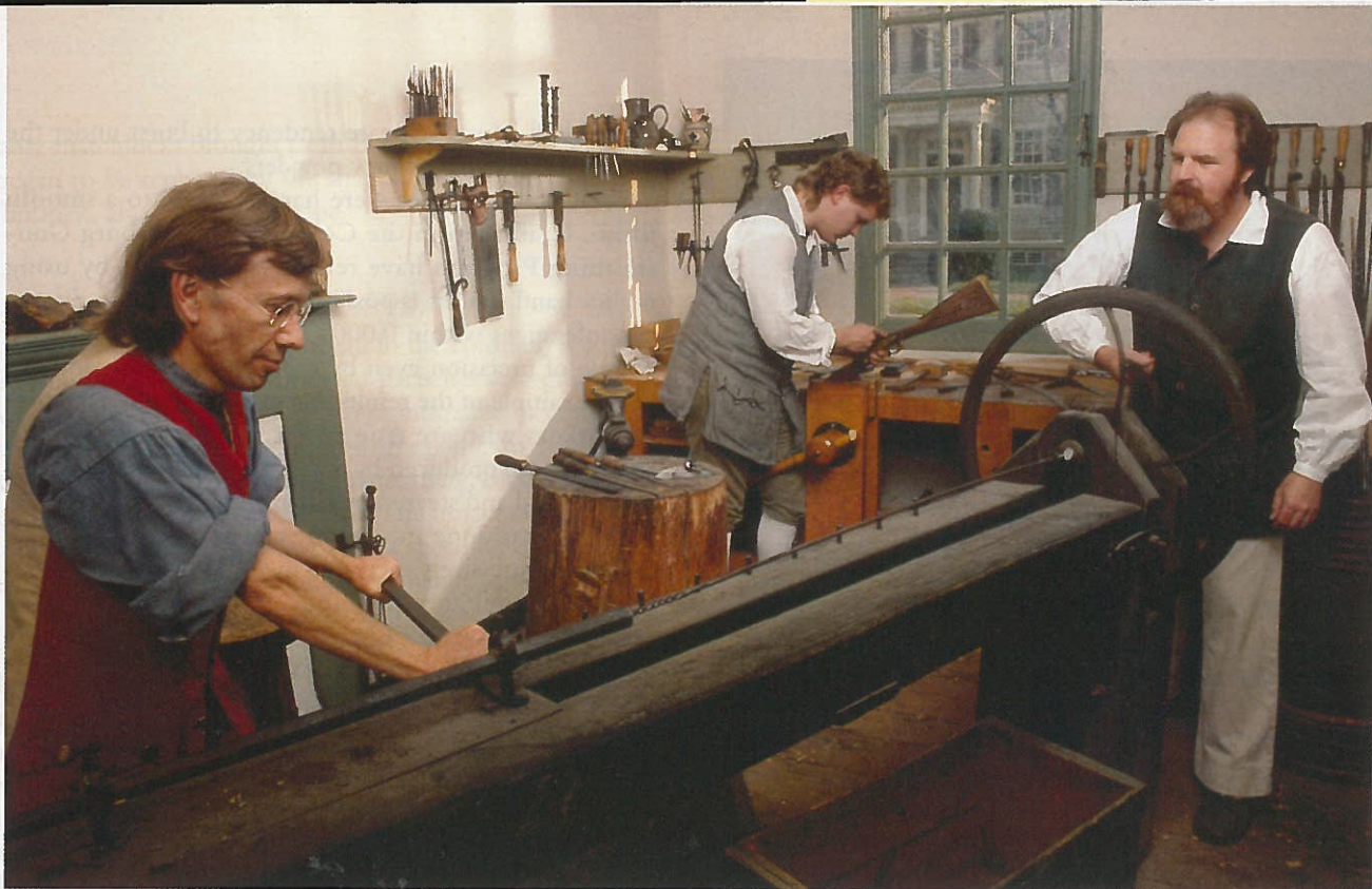
Craft drill: Master gunsmith George Suiter cranks as Richard Frazier, a journeyman, pushes a barrel to a drill bit. Alan Gutch (rear) stocks a rifle.
