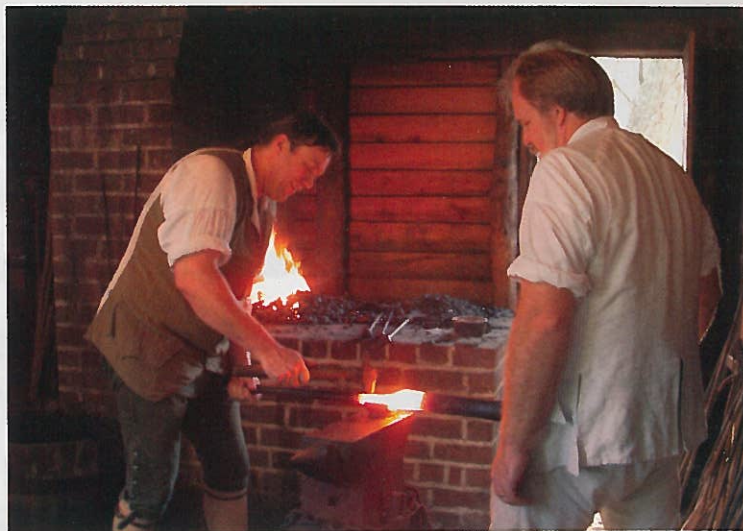
Barrel roll: Journeyman blacksmith Clay Smith works the barrel for a long rifle with the help of George Suiter at a forge in Colonial Williamsburg.
