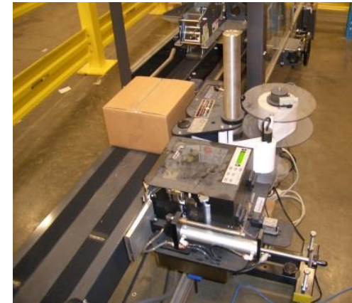
PLC-controlled Print & Apply Labeling
