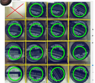
PC Screen shot of dunnage missing 1 part.
