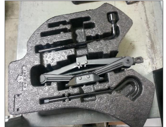
A Vision Sensor can detect the missing parts in this Jack Kit
