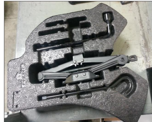
A USB Camera can ensure all slots in a container or kit are correctly filled
