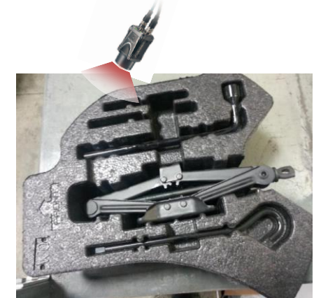
Vision can detect open slots in this Jack Kit
