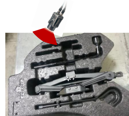
Vision can detect open slots in this Jack Kit
