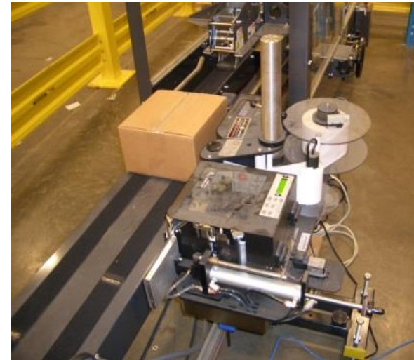
PLC-controlled Print & Apply Labeling
