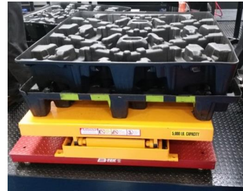
Weigh Scale Can Trigger Labels to Print
