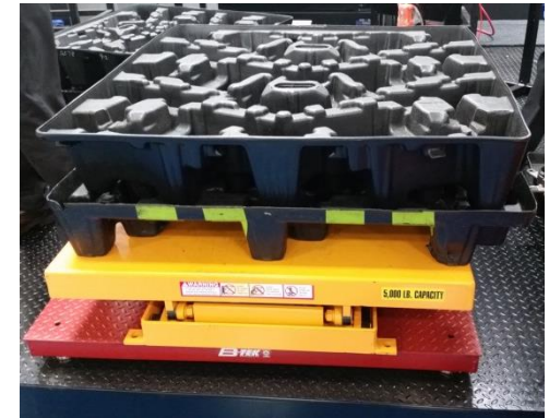
Weigh Scale Can Trigger Labels to Print
