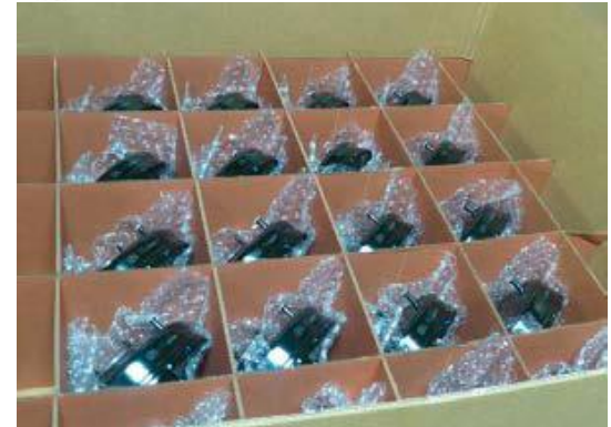
Validating all dunnage slots are filled correctly
