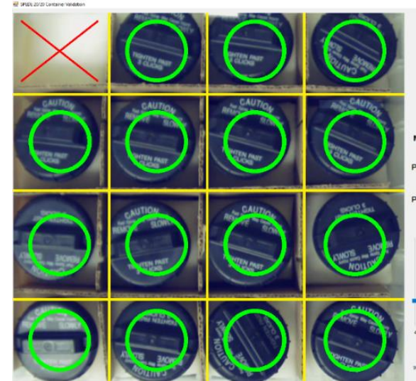
PC Screen shot of dunnage missing 1 part. No container label will print until slot is filled.
