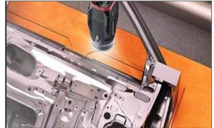
Vision sensors can validate parts for correctness, and ensure accurate pack counts
