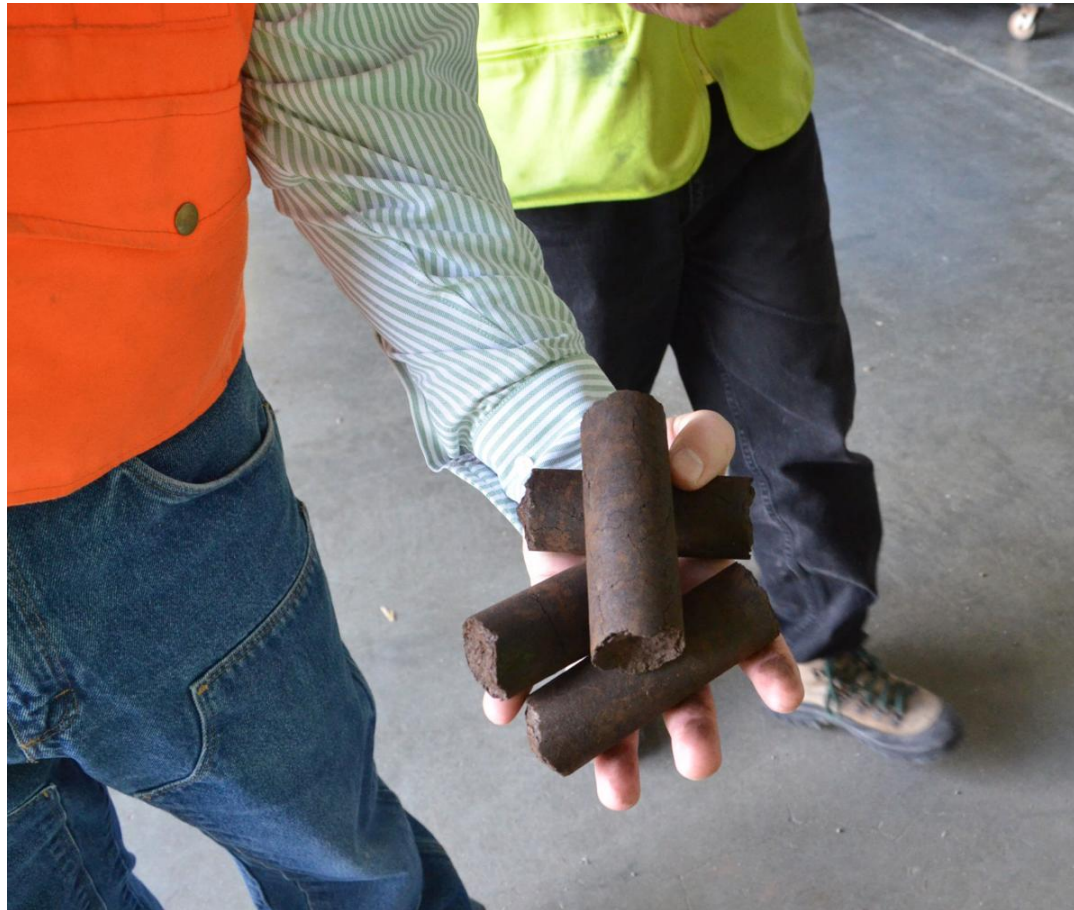
A handful of briquettes made from torrefied wood at a research facility in Louisville, Kentucky.
