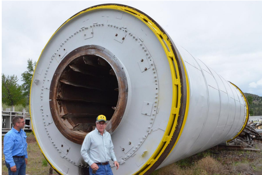
Matt Krumenauer, left, and Joe Koerner from Restoration Fuels LLC stand next to a triple-pass rotary dryer that will be repurposed for use as a torrefier kiln at the torrefaction plant in John Day.
