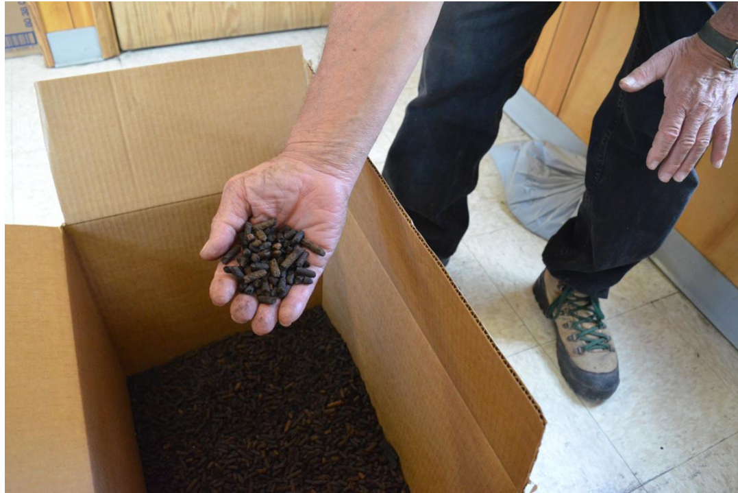
A handful of pellets made from torrefied wood at a research facility in Louisville, Kentucky.
