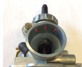
Slide to remain B&S stock unaltered. Slide cutaway to be measured on flat surface. .075 no go **Tech Tool A10**. All intake manifold fasteners to remain factory stock. The use of studs, etc. is illegal.
