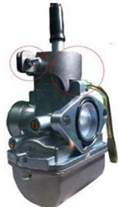
Optimization of the slide opening in Briggs & Stratton Kid Kart, Cadet, and Junior classes is permitted. The only allowable method of slide optimization is by removing material from the throttle cap area highlighted in RED. The use of multiple gaskets and/or machining of the slide is prohibited.
