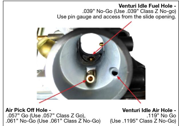
The "Slide Area" is the cylindrical space occupied by the carburetor slide as it moves up and down. Measurement surfaces of Tool A8 and A20 may not enter this space.
