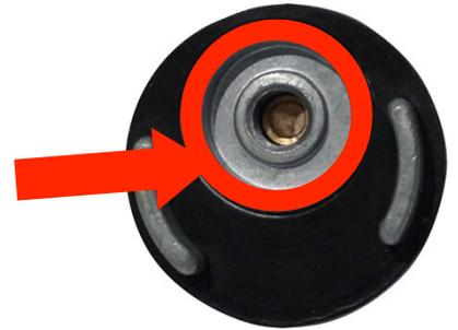
Slide opening must not exceed the appropriate No-Go specification as per class regulations. For information on slide optimization see video section at [www.BriggsRacing.com](http://www.BriggsRacing.com)
