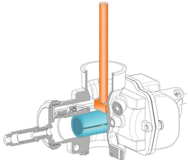
**NOTE: Slide openings should be measured only with the Briggs & Stratton slide tool listed on the tool reference chart.**
