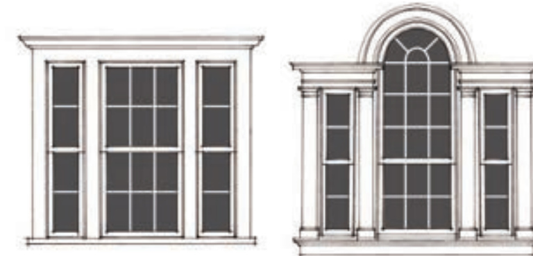
Triple paired windows are very common in this style, usually in special locations.
