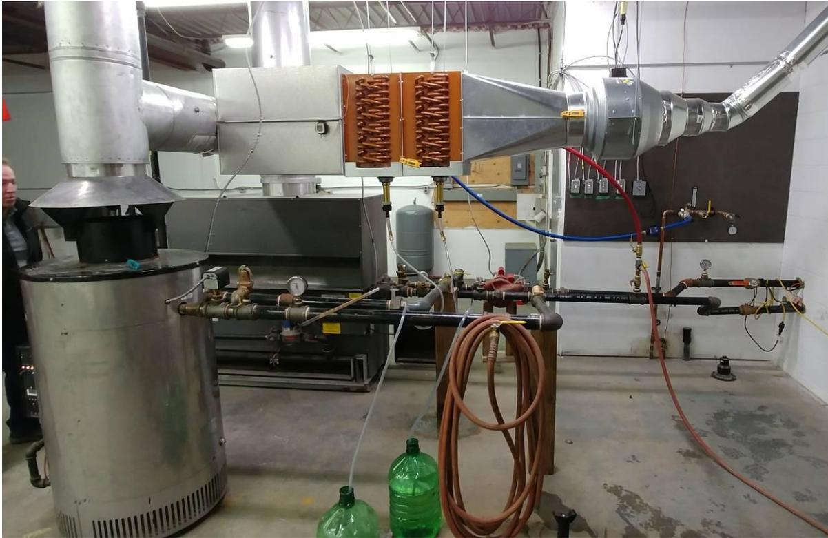
*Test setup including Camus boiler, venting, FGR heat exchanger, fan and connections.
