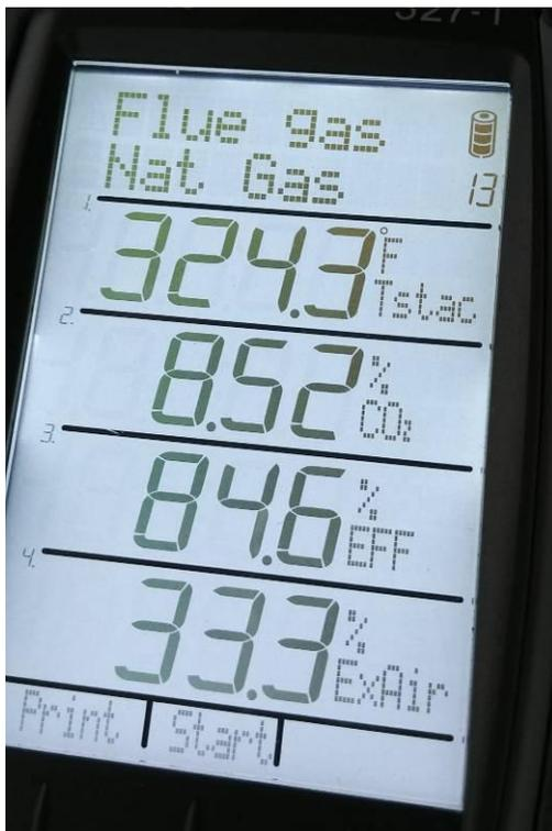
*Combustion analyzer output*
