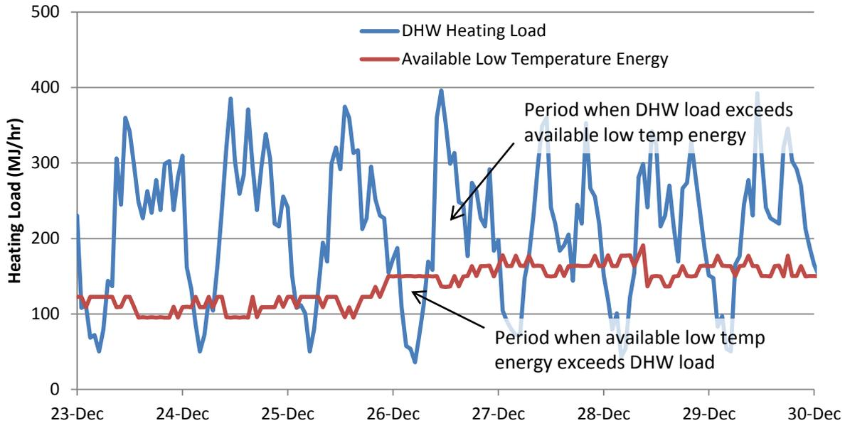
**Figure 2.** DHW heating load and available energy recovery from space heating system.
