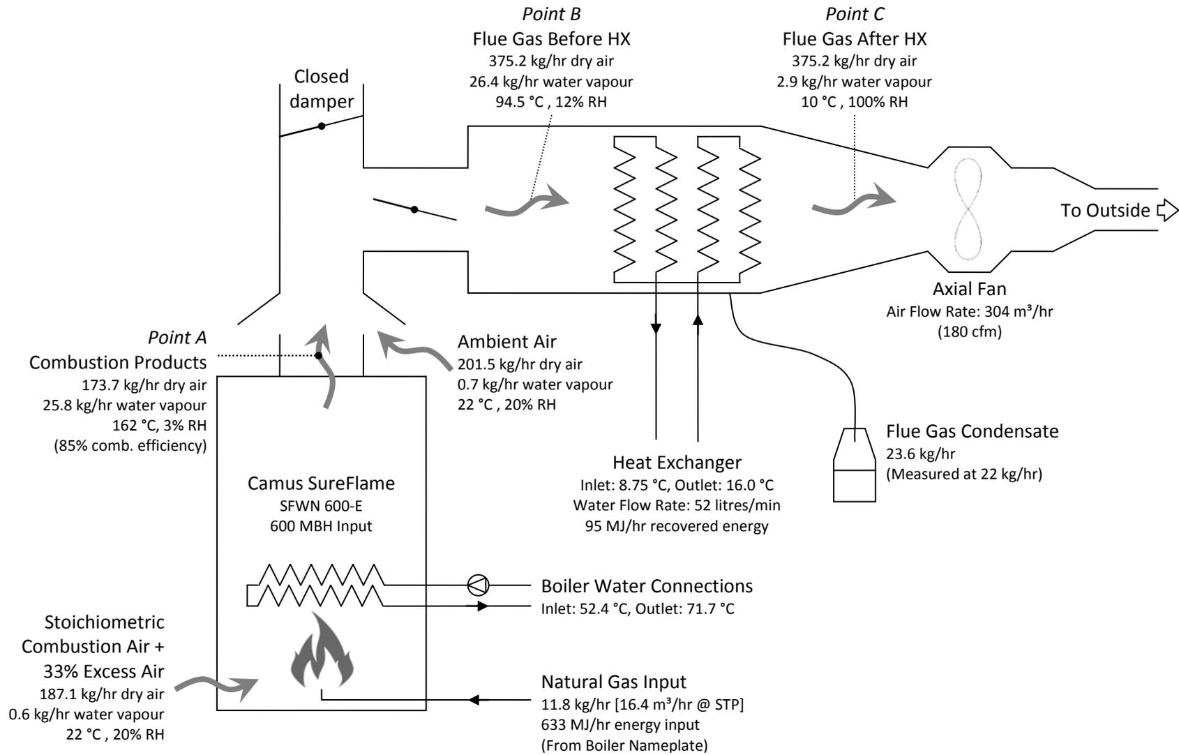
**Figure 1.** FGR system test configuration and values
