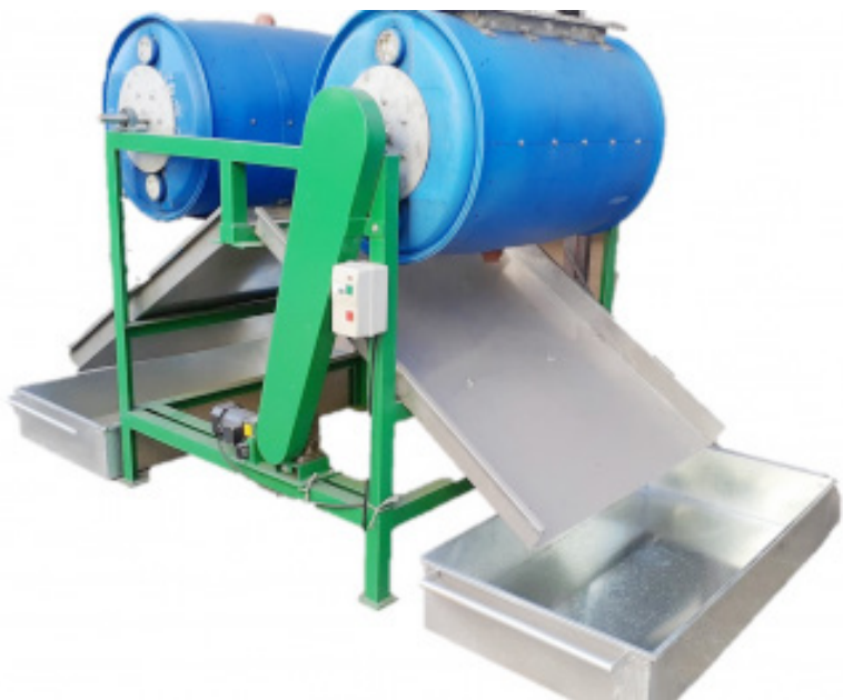
DUAL DRUM COMPOSTER. The Department of Science and Technology (DOST) is helping Cavite communities minimize their environmental footprint by introducing a device that turns garbage into fertilizer. Anna Marie Daigan, senior science research specialist at DOST's Cavite Field Office, said on Friday (May 10, 2024) this technology produces high-quality compost in a short time. (Photo courtesy of DOST Industrial Technology Development Institute)
