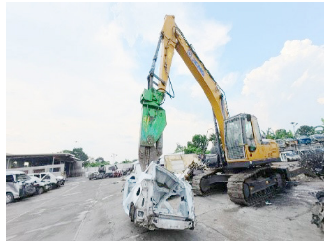
RESPONSIBLE DISPOSAL An excavator fitted with a hydraulic shear attachment dismantles an end-of-life vehicle (ELV) at Standard Insurance’s ELV dismantling facility. PHOTO FROM TMP
