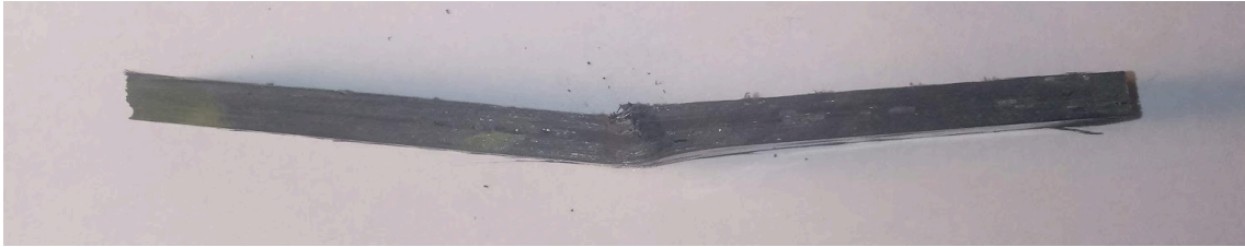
Figure 3. Sample 1 post-test did not reach failure, but underwent significant plastic deformation in the form of compression (top face), tension (bottom face), and bulging.
