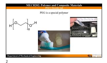
**MECH202: Polymer and Composite Materials** Lab Objectives - Test for the viscosities of PEG at different molecular - Graph the intrinsic viscosity for each molecular weight vs is molecular weight - Find the alpha value of the solution and check tabulated values to see if it is correct Department of Mechanical Engineering PACIFI
