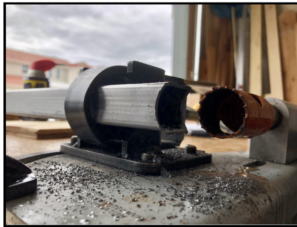
Figure 5: Square tube being cut with tube notcher
