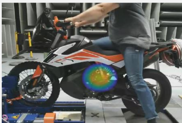
Figure 2 High accuracy localisation of low frequency sound emissions from a motorcycle operated at full throttle on a roller dyno. Acoustic images are recorded with same dynamic range of 3dB.
