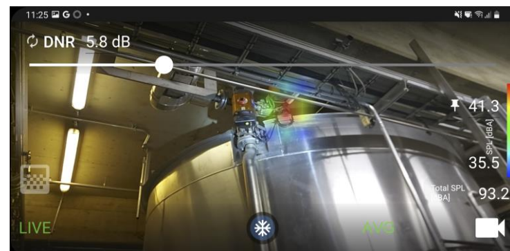
SPL AT 1M 50.8DB DISTANCE 3M SPL AT MEASUREMENT DISTANCE 41.3DB
