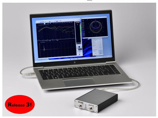
**CLIO Pocket** is an Electro-Acoustical Multi-Platform Personal measurement system.
