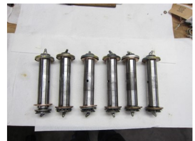
H-25 blade pins ready to install
