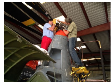
Checking H-25 blade lock pins
