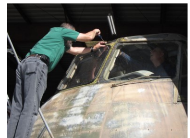
Replacing H-37 windscreen
