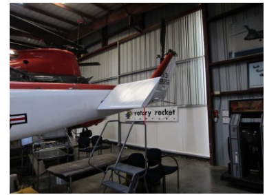
Repainted H-1N stab replaced
