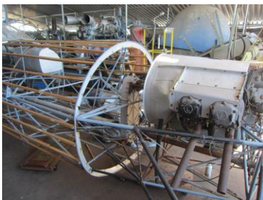
Engine firewall removed
