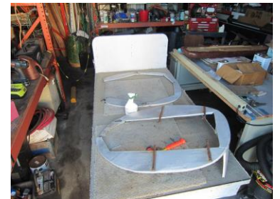
Fuselage frames repaired
