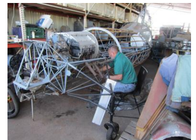
Fuselage corrosion removal
