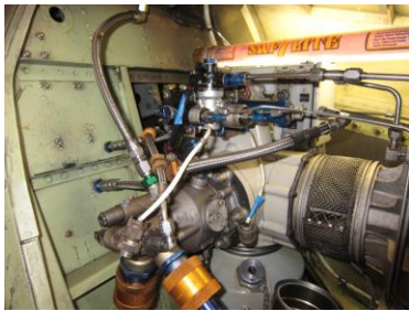
Removing APP fuel control
