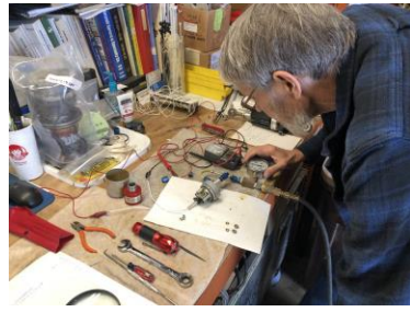
Testing oil pressure switch
