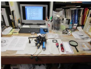
Working on APP fuel control
