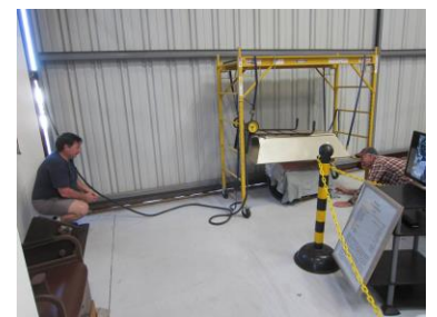
Oven forming cockpit window
