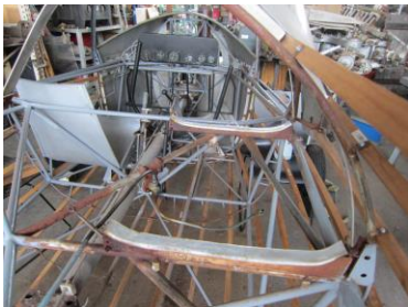
Fuel tank removed
