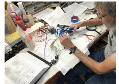
Building a new wiring harness
