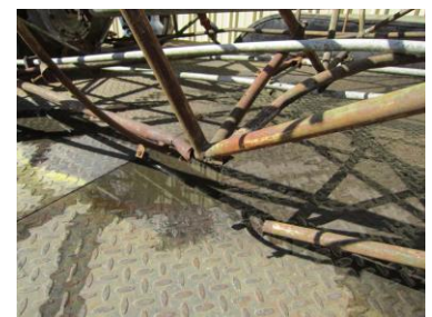
DL-125 broken fuselage tube
