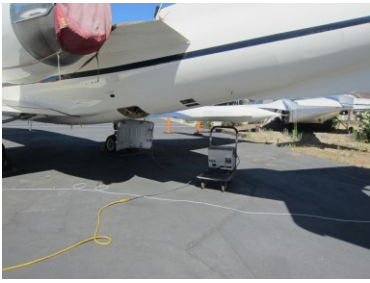
Charging Lear Jet battery
