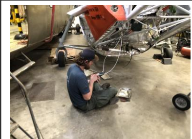
Wiring the HRP external power
