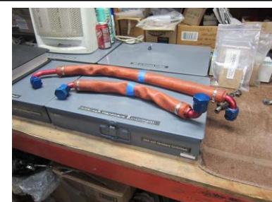
Engine fuel hoses removed
