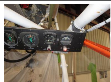
HRP voltage gauge and light
