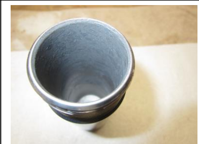
Pitting in Huey ground wheels
