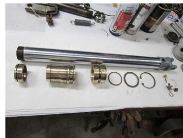
HRP NLG strut restored
