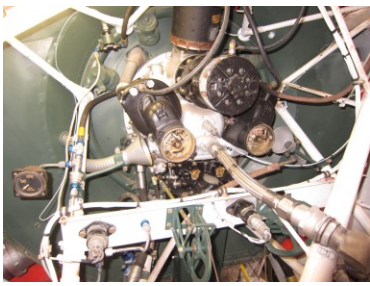
HRP magneto cooling tubes
