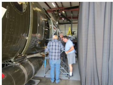
Relocating H-21 entrance steps
