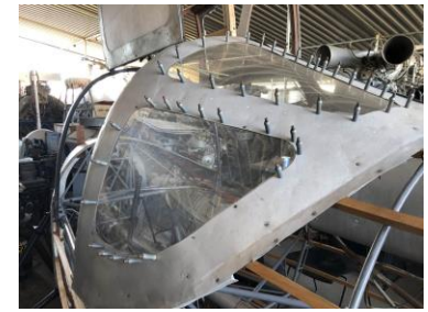
DL-125 rear windows in place
