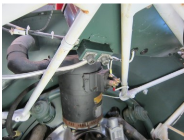
HRP ignition switch
