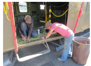
Stripping the H-37 entry deck
