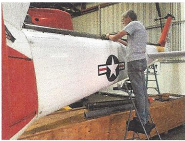
The HH-1N tail rotor drive shaft
