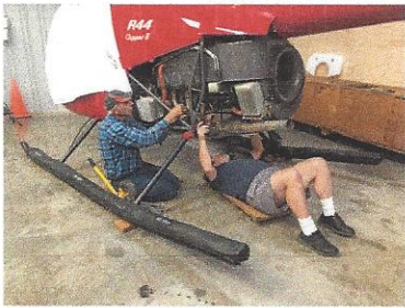
Checking exhaust alignment
