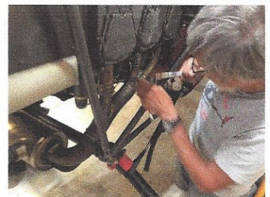
Securing the exhaust manifold
