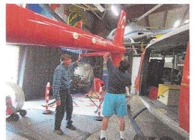
Checking the R44 tail alignment
