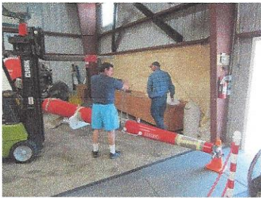
Lifting the R44 tailboom
