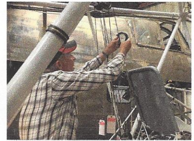
HRP control cable tensioning
