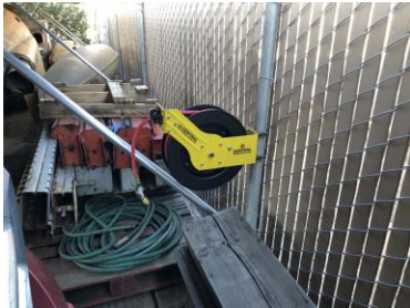
Compressor hose reel
