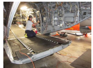
Repairing a ramp actuator leak
