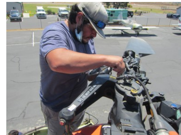
Eddy Current head inspection
