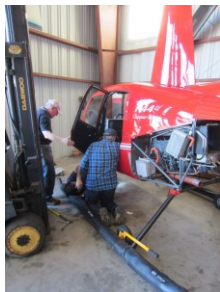
Skids bolted on
