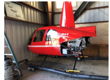
R44 fuselage and skids are one
