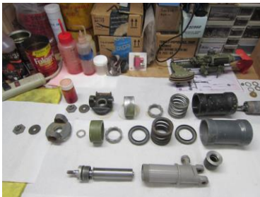
Disassemble the dampers
