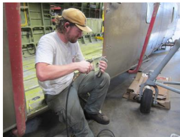
Cleaning a control bellcrank
