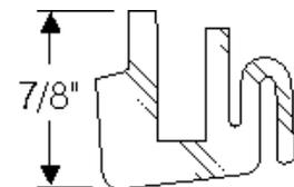
**805452:** Windshield seal for 1941-46 Studebaker cars with stainless molding. This is not identical but will work. Most windshield gaskets of this period are available as unitized and correct gaskets. See our other rubber listings by application.
