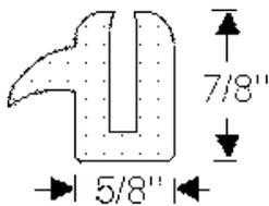
**818852:** Used as both windshield and back glass seal with 1/4" glass, has thick weather-lip and notch for bead reveal molding if required.
