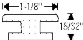
**809852:** Universal gasket, for divided windshield center-post. Depending on your application, trimming may be required, combines inner and outer gasket in one piece. Available in 20 inch length only.
