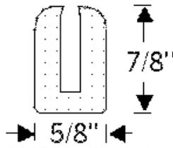
**819252:** Seal channel used for windshield, backglass and stationary quarter windows. For windows with chrom reveal molding. Plain compression channel for ¼” glass. Found on many makes in the 1930’s.
