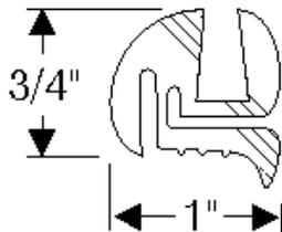
**801252:** Cross section of windshield gasket used in most post-war Studebakers, available only in lengths of 12 feet. Can be mitered and glued for sharp corners.
