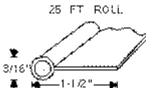
**800587X25:** Fender welt between fenders and body. Bead is flexible and paintable. Minimum 25 foot roll.
