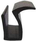
**807557:** Glass setting channel. Holds 1/4" glass into steel glass carrier channel and incorporates a weather-lip. Dimensions: 3/8" width at bottom, 11/16" deep.
