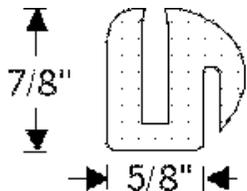
**819052:** Used as a seal for windshields, back glass, and stationary quarter window. Has a thick weather-lip and a notch for bead reveal molding if required. For ¼” glass.
