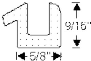
**819552:** Windshield seal. Used with or without chrome reveal molding. Channel for ¼” glass with lip for attaching beaded molding. Frequently used on many makes in later 1920’s thru 1930’s.
