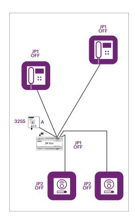
INDOOR: The kit allows a maximum of 3 terminals (the included one and 2 additional ones). Depending on the type of cable and distances, an additional power supply (ref. 4825), line adaptor ref. 3255 and/or regenerators might be required.
