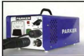
B100 - A.C. Contour Probe. Our most economical. May be ordered with the Y400 Yoke Light at extra cost.
